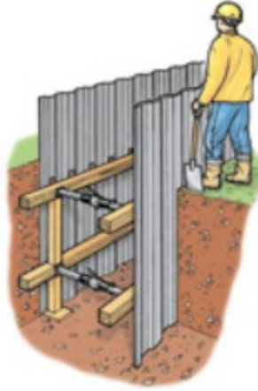
Trench sheets with timber walings, screw props, puncheons and sole plates
